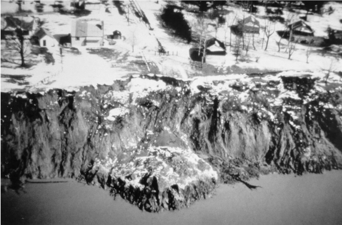
Figure III-5-21. A rotational bluff failure along the north central shore of Lake Erie
